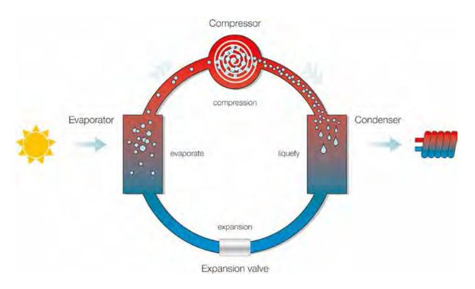
Heat pump water heater extracts energy from the air or other heat source and uses it to heat water. It uses 1 time power to drive the compressor and brings 4.3 times heat to the water, this is what we called coefficient of performance(COP). With COP up to 4.3.
